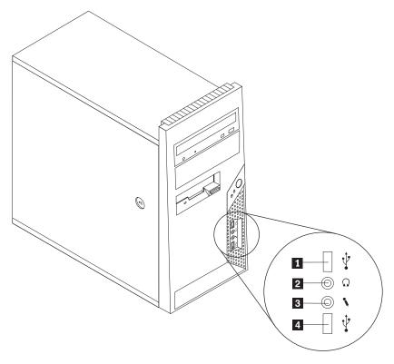
Figure 1. Front connector locations
